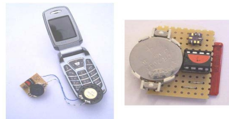
Fig. 1 Proof of concept prototype connected to a mobile phone.
